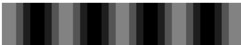
Fig.2: Pattern formed on screen showing differing intensities caused by light wave interference
